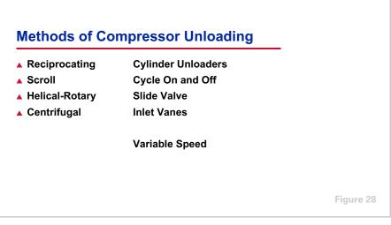
Capacity control is commonly accomplished by unloading the compressor. The method used for unloading generally depends on the type of compressor.
